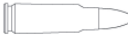
FIG. 564 Cal. .22 High Velocity Ball Cartridge with 20.6 gr. Hollow-Point Bullet for Personal Defense Weapon (from specimen headstamped W C C 6 3)
