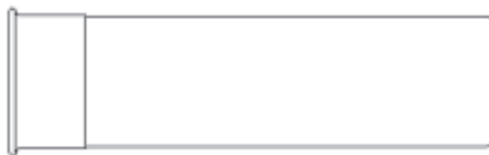
FIG. 759. 28 Gauge Blank for M1A1 Spotting Charge for M38A2 100 lb. Practice Bomb (from specimen headstamped WESTERN MADE IN U.S.A. NQ 28 XPERT).
